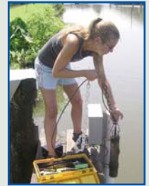
Graduate student Laurie Rodrigue deploys a meter that will measure the dissolved oxygen in Bayou Terrebonne.
