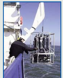
An oceanographic instrument called a CTD is lowered into the Gulf of Mexico during a research cruise.
